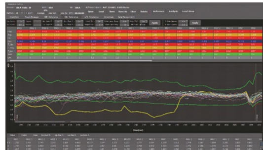
〈 Example of poor welding quality 〉
